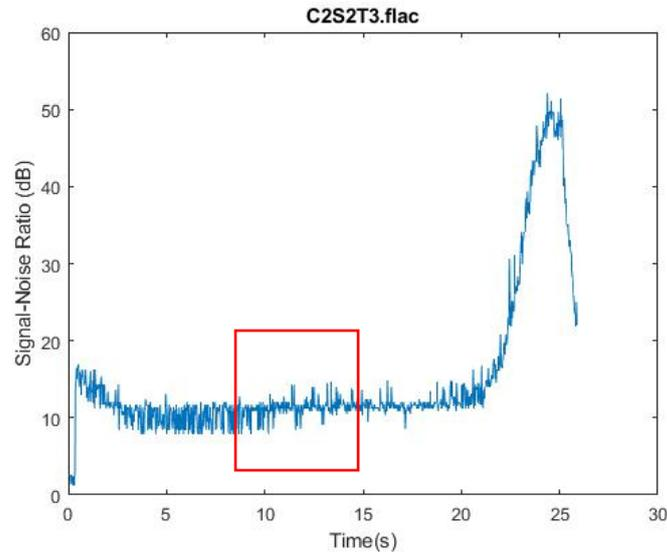
**Figure 2 SNR plot of a sample signal**
