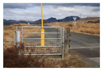
Access through any bypass gate should be unrestricted in both directions. The yellow barrier post on the far side of this self-closing bridlegate makes it difficult for horses and users of mobility vehicles to negotiate the gate. If you come across a problem such as this, contact the landowner or manager, local access officer or your local equestrian access group to discuss appropriate action to remedy the problem.
